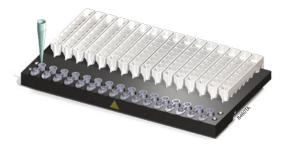
Figure 2. The Elution Tubes are placed in the front of the Maxwell  $^{\rm B}$  16 LEV Cartridge Rack, and 50 $\mu$ l of Nuclease-Free Water is dispensed into each tube.
