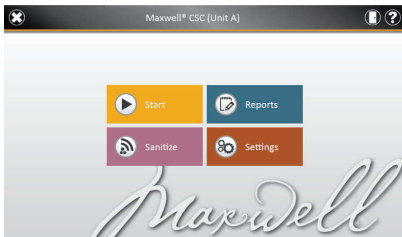
Figure 30. Maxwell® CSC Home screen. Selecting Settings opens the Maxwell® CSC Settings screen from which bar code entry options can be configured.
