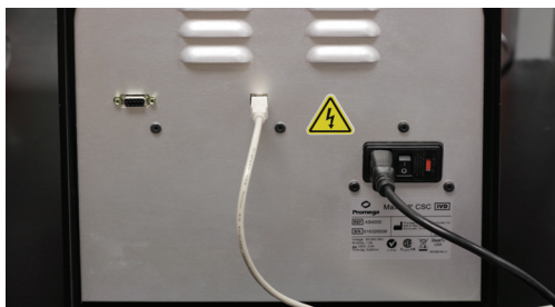
Figure 15. Connect the Tablet PC to the back of the Maxwell® CSC Instrument.
