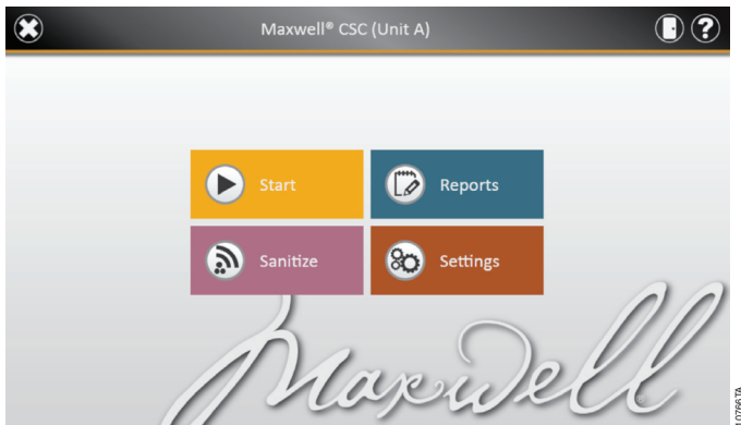
Figure 65. Maxwell® CSC Home screen. Selecting 'Reports' opens the Maxwell® CSC Reports screen from which extraction reports from all protocol runs can be viewed.
