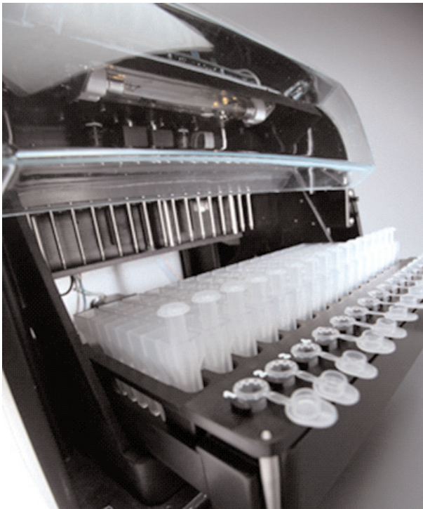
Figure 4. Magnetic assembly components and platform. The hardware components inside the Maxwell® CSC Instrument. The magnet and plunger bars, which are used for sample processing, and the platform containing the deck tray are evident.
